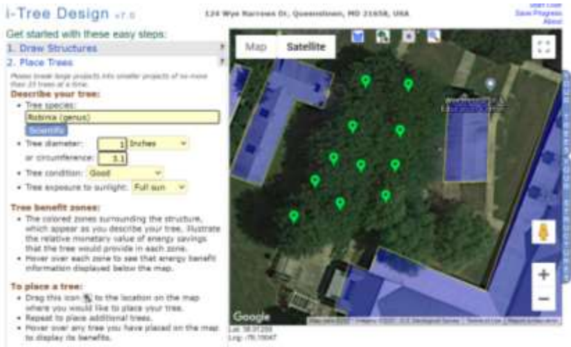
Figure 7 – I-Tree Design overview of area between buildings + Robinia sp pins. Assumes trees in good condition.
